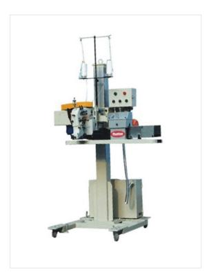
The automatic bag folding and sewing machine adopts photoelectric control and can automatically and continuously complete folding, stitching, trimming and braiding of the mouths of kraft paper or plastic woven bags. Its air supply system realizes thread trimming, cutting and oil mist lubrication. The height of the machine can be adjusted according to the bag size.
